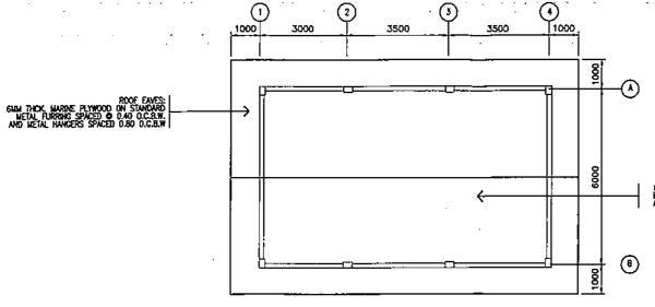
6MM THCK, MARINE PLYWOOD ON STANDARD METAL FURRING SPACED © 0.40 O.C.B.W. AND METAL HANGERS SPACED 0.80 O.C.B.W
